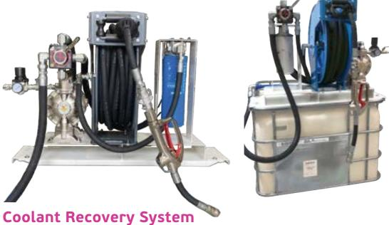
IBC Mounted Coolant Recovery
